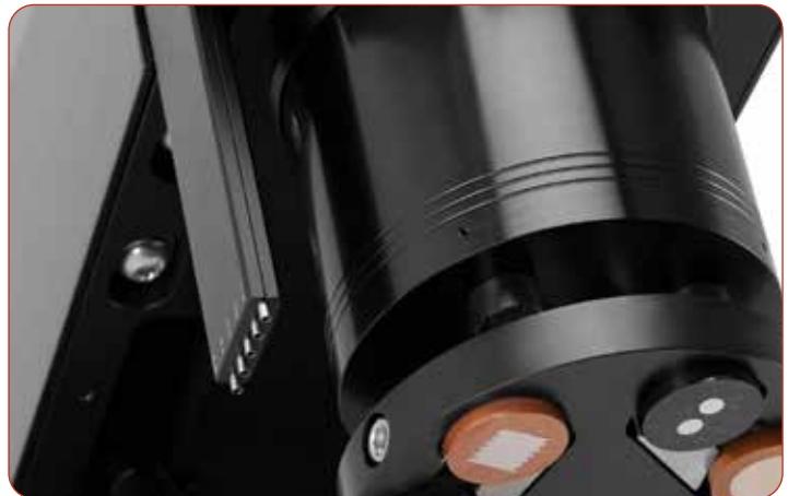
ID-5x™ dispensing nozzles in a pivoting manifold
