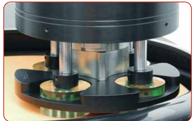
PH-4™ individual force configuration: four (4) individual pistons apply force to each mount (1.5" mounts shown).
